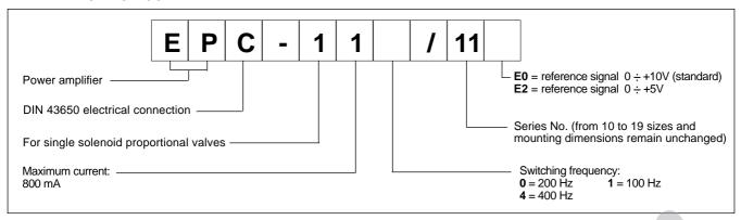
The EPC unit is a miniaturised electronic control unit for open loop proportional valves, designed in plug version in compliance with DIN 43650, for direct mounting on the valve solenoid.
